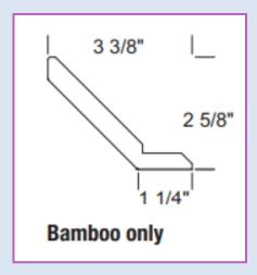
Medium Straight Angle Crown Moulding is only available in 96" length with attached cleat. It's a great addition to the sleek lines of Jules Bamboo.
